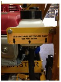
The Razer has the newest hydrostatic transaxle that requires no hydraulic fluid. The Razer only requires 20-50 Motor Oil, which should be filled to the bottom of the reservoir mounting bracket.
