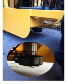
These ports service both actuator support bearings and both crank shaft bearings. Actuator Rod Bearing is accessed from under the Razer frame. Grease these points EVERY 10 HOURS OF OPERATION. Grease Actuator Lever AS NEEDED.
